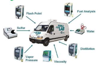
Also Available as a Mobile Environmetal Testing Laboratory or for other applications.
